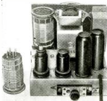
A rear view of the midget "metal-tube" all-waver, which uses plug-in coils to cover the various bands.
