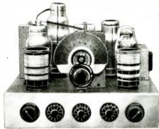
The revamped 2-volt superhet, with regeneration feature added.
